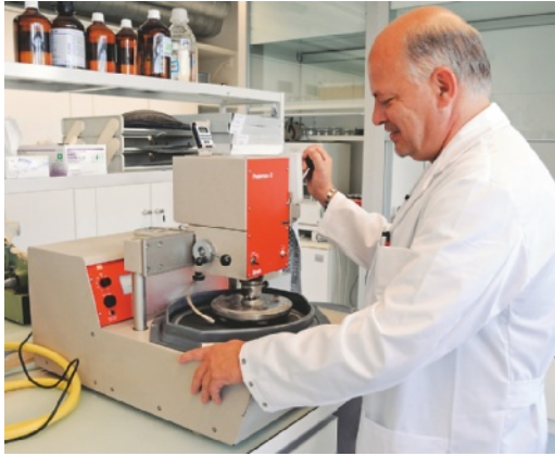
Fig 10-10 The ground sections are glued on a Plexiglas slab and ground to a final thickness of 80 to 100 \mu\text{m} .
